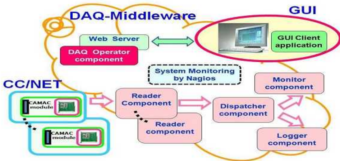
Figure 4. An entire block diagram of the DAQ System for the CC/NET.
