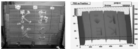
Fig.4. 2-D imaging data obtained by forty PSD detectors. The left figure is a picture of PSD detectors with the characters "KEK!" using cadmium plates. The right figure shows 2-D imaging data obtained by a neutron beam scattered by a polyethylene block.
