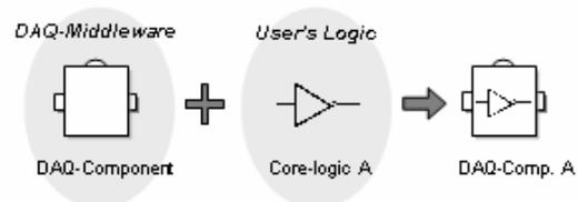
Fig. 2. DAQ-Component and its core-logic.
