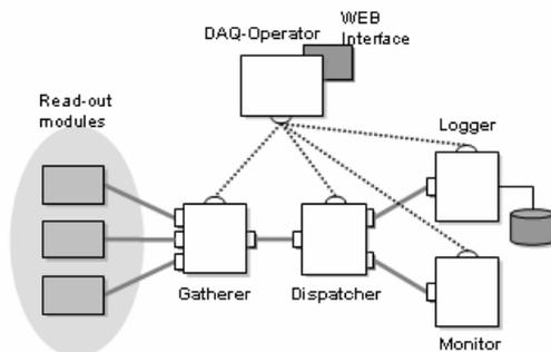
Fig. 1. Fundamental DAQ-Components of DAQ-Middleware. This figure shows the fundamental DAQ-Components and one of their configurations. Solid lines show data paths and dotted lines show command/status paths.
