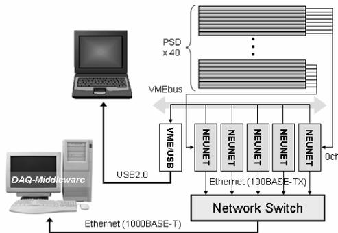
Fig. 3. Schematics of the DAQ setup for the beam-test.
